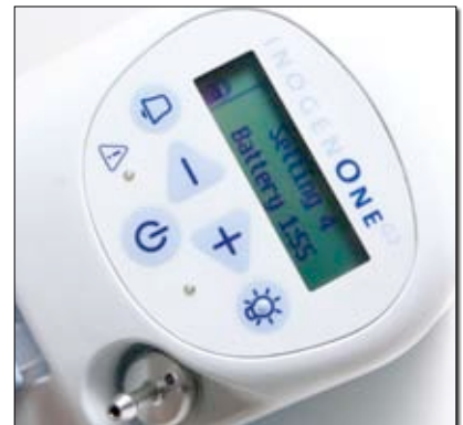
A control panel shows the level setting and battery life remaining, among other messages.
